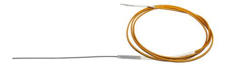
PCS Company's Hot Sprue Bushing Thermocouples are all J-type. They are 1mm in diameter and come in lengths to it PCS Hot Sprue Bushings. These thermocouples are designed to be a backup to the intregal thermocouple found in the body heaters.
